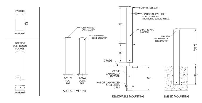
B-2 Bollards shown above in 5" pipe, also available in 8" dia. and in 30", 36", 42", and 48" heights, removable bollard receivers sold separately.
